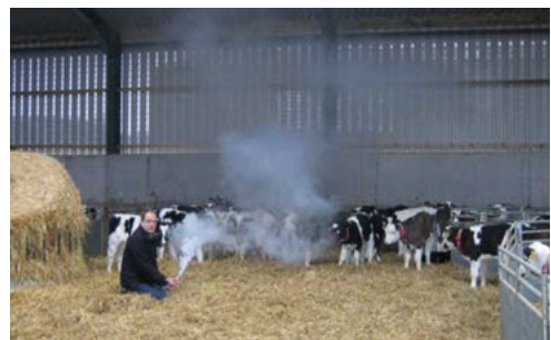
Figure 1. Use of a smoke test to show the flow of air within the building
