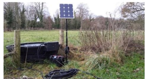
Figure 7: Photovoltaic pump
